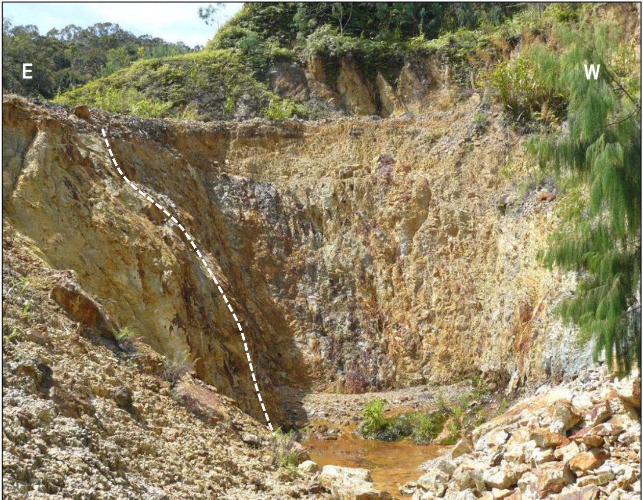
Figure 8-5: View of the Sinivit South pit in February 2025, looking south-southwest. Note the exposure of the steeply west dipping, undulating, and 020° striking Wild Dog structure on the east side of the pit face (dashed line), with pronounced argillic-phyllitic-silicic alteration extending into both the footwall and (predominantly) hanging wall. Photograph taken by the QP (Frank Bierlein).
