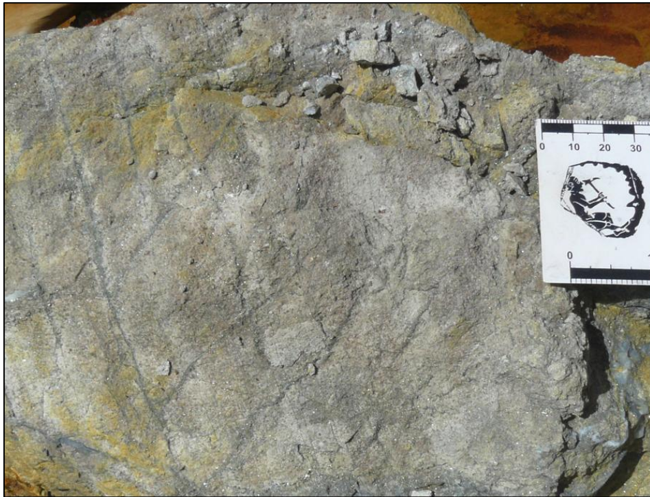
Figure 7-6: Criss-crossing Type III veins in the floor of the Sinivit South Pit (photograph taken by the QP Frank Bierlein in February 2025).
