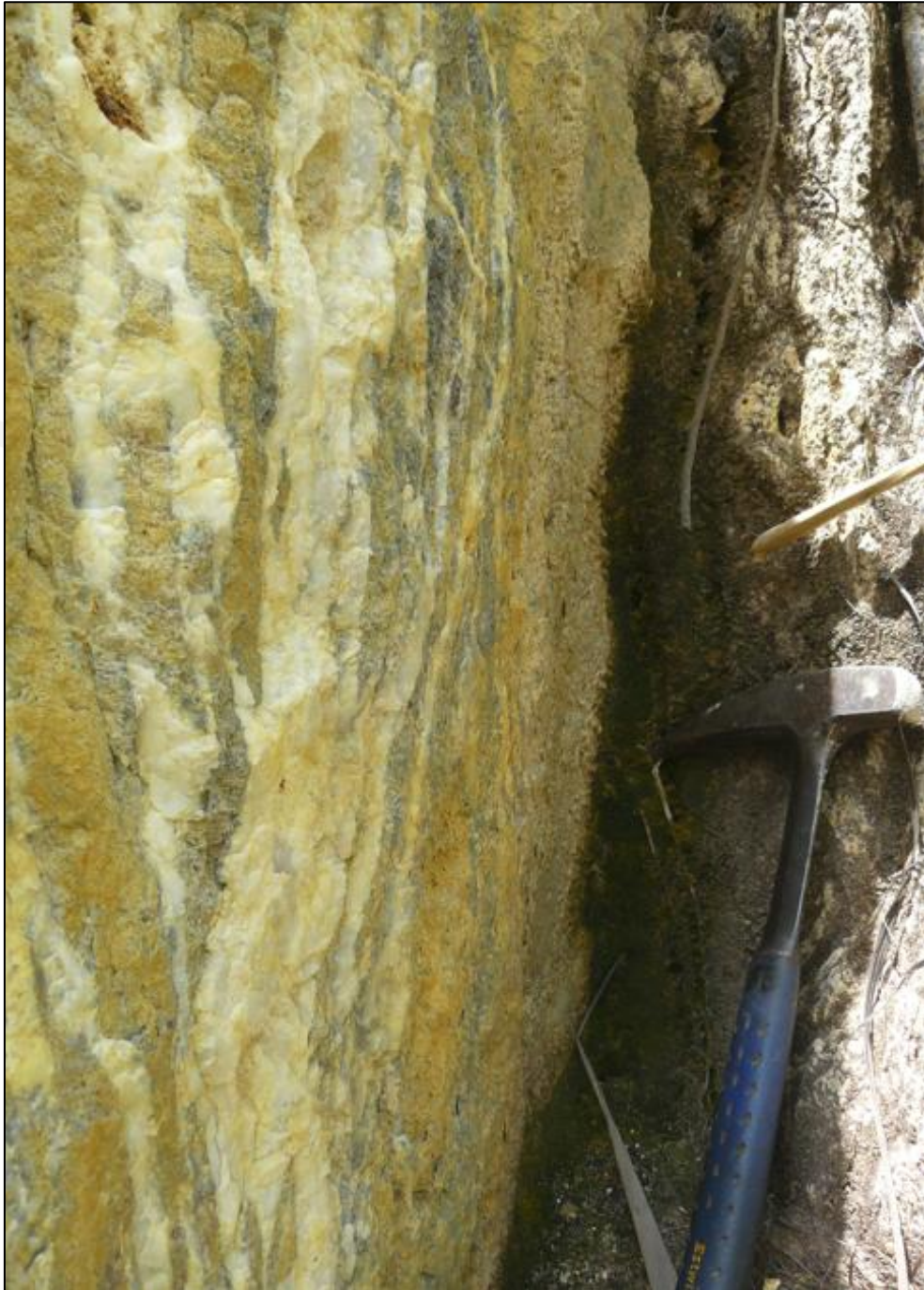
Figure 8-6: Example of north-northwest trending, sub-vertical set of quartz tension veins in the South Sinivit pit, truncated by an east to west trending dextral strike-slip fault. Photograph taken by the QP (Frank Bierlein) in February 2025.
