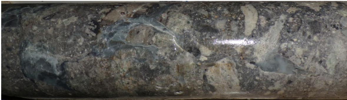
WDG-02 79m hydrothermal breccia with dark sulphidic quartz.
