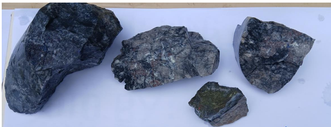
WDG-04 64.6m broken up core with strongly mineralized black sulphidic silica, chalcopryite and bornite.
