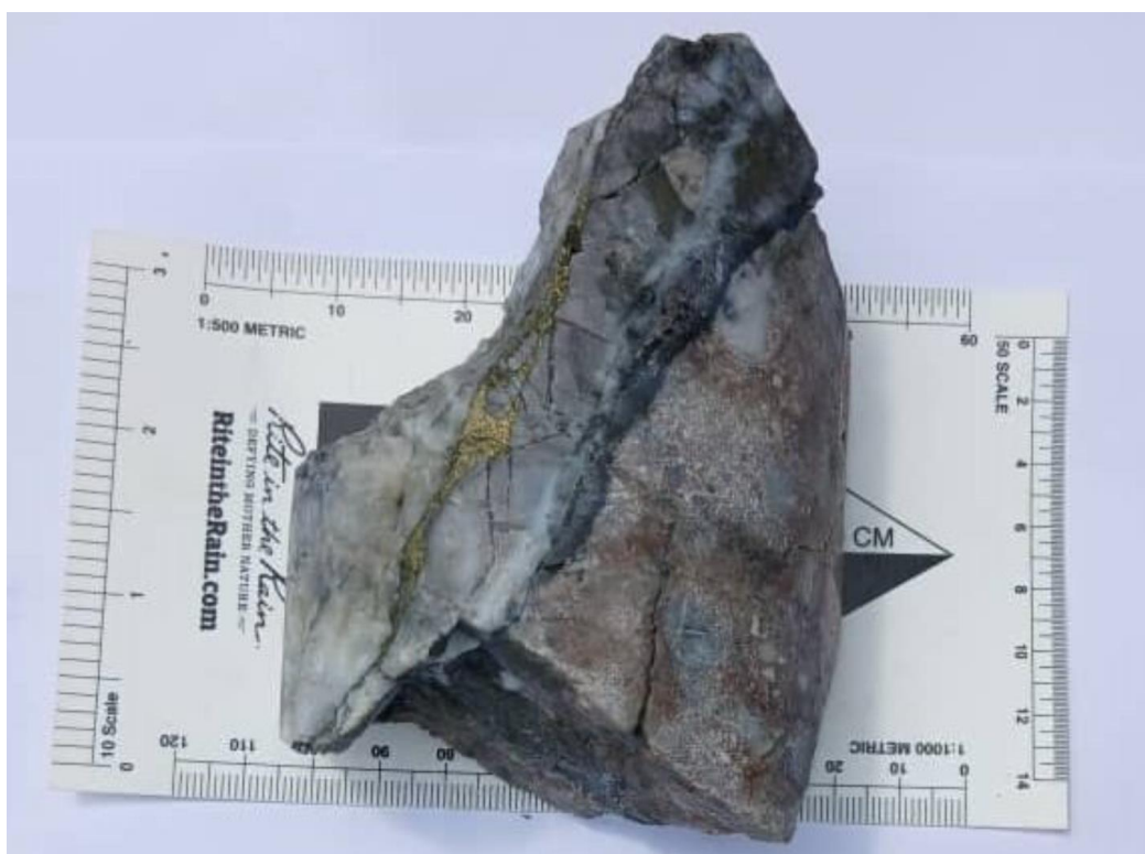
WDG-04 64.0m Fine-grained epithermal quartz vein hosted within brecciated and silicified wall rock. The vein is distinctly selvaged by grey to black sulphidic silica, interpreted to be chalcadonic in part, with coarse-grained chalcopryite (cpy) infill visible along fractures and vein margins. This texture is consistent with multiphase epithermal fluid pulses and is representative of the mineralised structures intersected in WDG-004 within the Wild Dog vein system.
