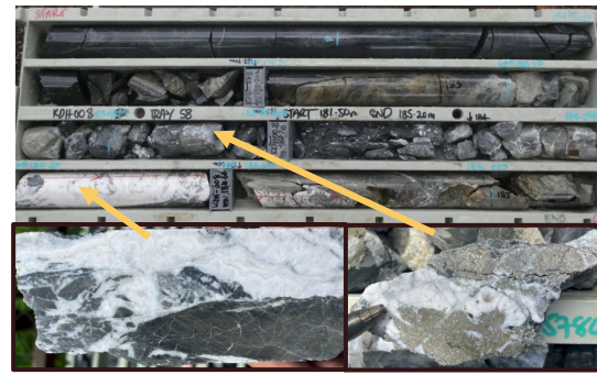
KDH-08 Core Photograph: 181.5 – 185.2m; Hydrothermal breccia with Quartz-Carbonate vein and semi-massive pyrite
