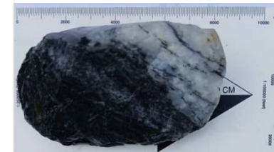
WDG-04 65.2m well-banded epithermal vein assaying 103 g/t Au
