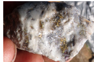
WDG-02 64-67m coarse chalcopyrite and bornite
