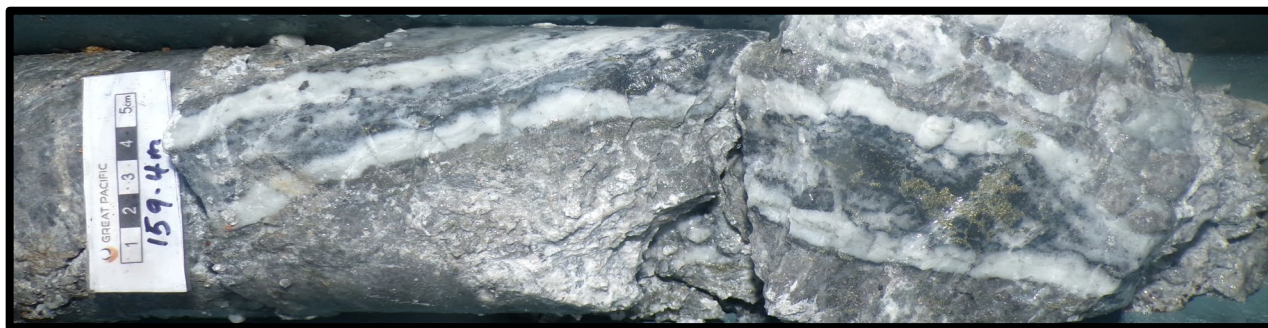
Photo of WDG-07 drill core from 159.4 m, showing strongly banded colloform and crustiform quartz with dark sulphides, including visible chalcopyrite and bornite. The outer margins of the vein exhibit grey-white chalcadonic silica with multiple generations of mineralisation overprinting inward from the vein margins.
