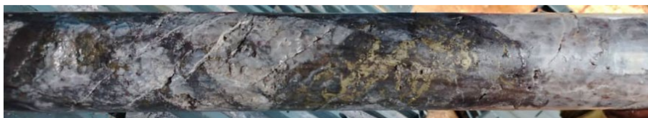
Photo of WDG-08 drill core at 156 meters showing semi-massive sulphides with visible chalcopyrite and bornite. Assays are pending for this interval, and visual observations should not be considered a proxy for grade.
