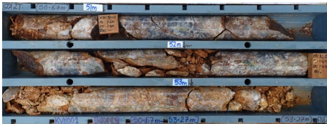
Figure 5: KVVH-01 50.67-53.27m core photo. Oxidized hydrothermal quartz breccia with zone of dark sulphides
