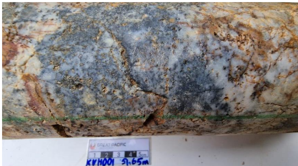
Figure 4: KVH-01 close-up at 51.65m. Oxidized hydrothermal quartz breccia with black sulphidic silica infill
