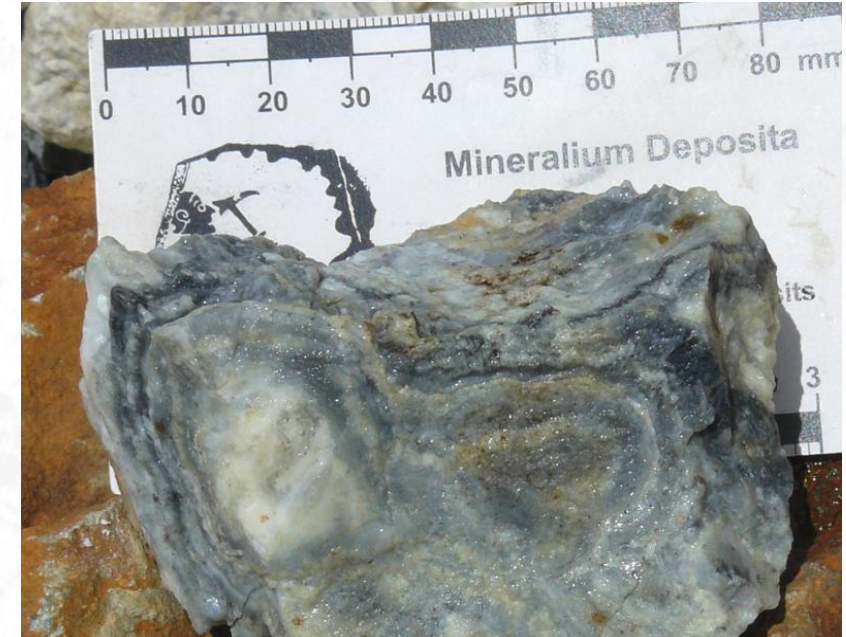
Example of 020°-trending, vertical Type I vein in the Sinivit Central pit and crustiform chalcedonic silica bands in Type IV veins from the Central Sinivit pit (photograph taken by the QP Frank Bierlein in February 2025).
