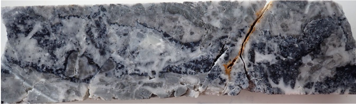
Figure 3: KVH-01 core photograph (67.4 m): Bands of dark sulphides within quartz breccia.
