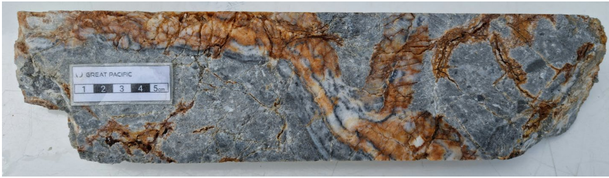
Figure 6: KVH-01 core photograph (81.0 m): hydrothermal quartz breccia with partial oxidation and thin bands of black sulphides.
