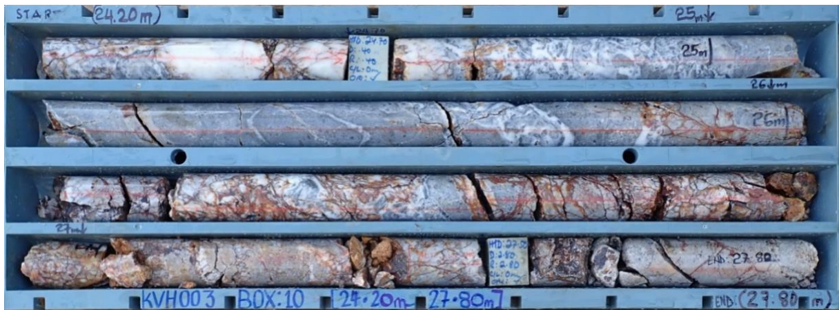
Figure 4: Drill core from the Kavasuki hole KVH-03 (24.2-27.8 m) showing intense silica flooding and multi-phase quartz veining within hydrothermally altered host rock.
