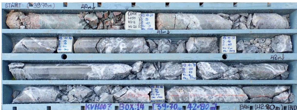
Figure 5: Drill core from the Kavasuki hole KVH-03 (39.7-42.8 m) showing intense silica flooding and multi-phase quartz veining within hydrothermally altered host rock.
