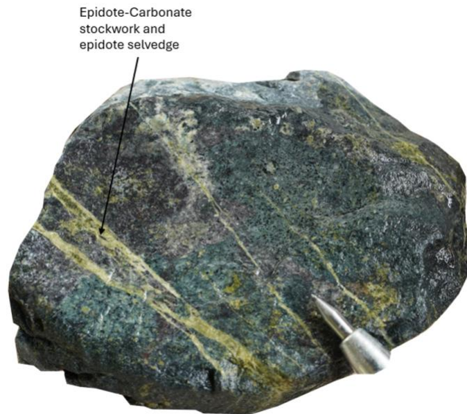
Figure 7: Propylitic-altered volcanic host rock from the Kasie Ridge drill hole showing epidote–carbonate–quartz stockwork veining with epidote selvages from 50-56 m.
