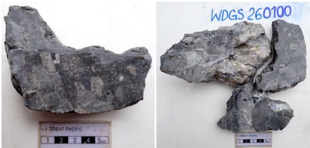
Figure 6: Rock-chip sample WDGs260100 from the Magiabe West Vein showing a fault-hosted, clay-filled zone with disseminated to locally massive pyrite, bornite, and chalcopyrite ( 90.9 g/t Au, 30 g/t Ag, 0.45% Cu ).
