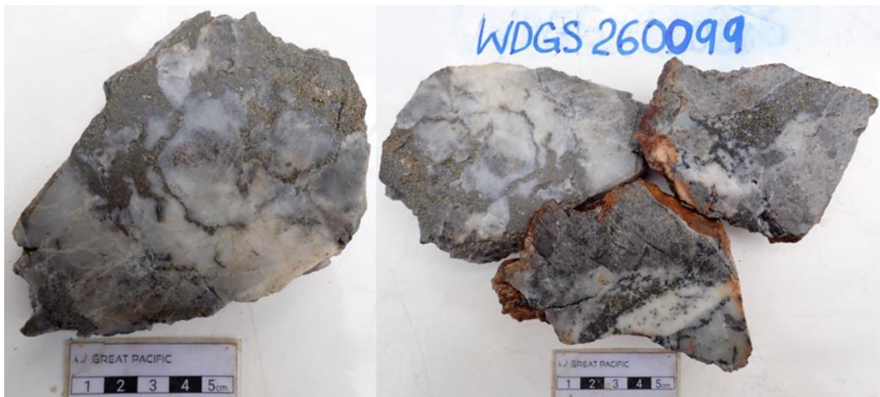
Figure 5: Rock-chip sample WDGs260099 from the Magiabe West Vein showing a clay-filled fault zone with disseminated to locally massive pyrite, bornite and chalcopyrite ( 41.1 g/t Au, 31 g/t Ag, 4.3% Cu ).
