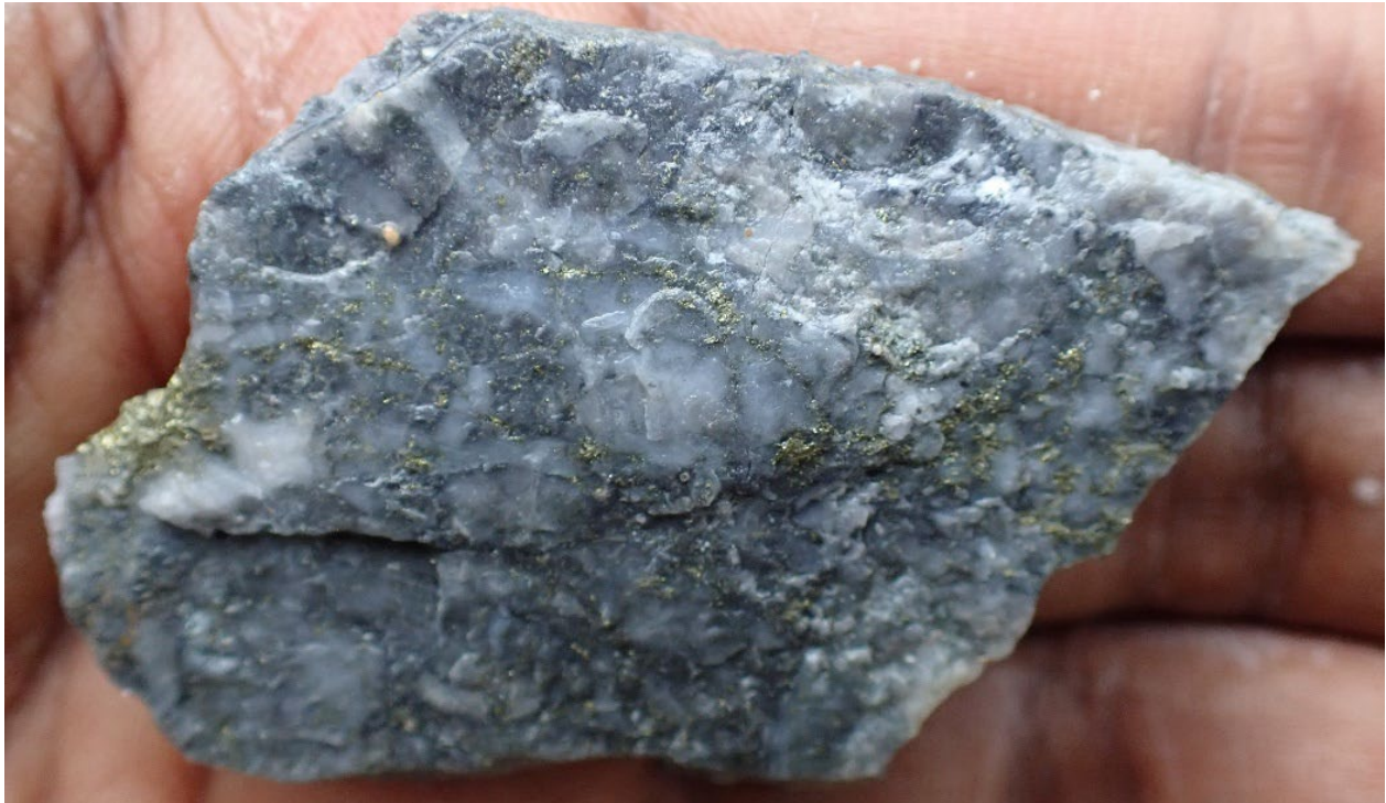
Figure 4: Close-up photograph of sulphide-bearing quartz vein material (KVH-03; 48.7m), showing fine disseminated sulphides within silica flooding and brecciated quartz (WDDH002686: 46.6 g/t Au, 35.0 g/t Ag and 0.58% Cu).
