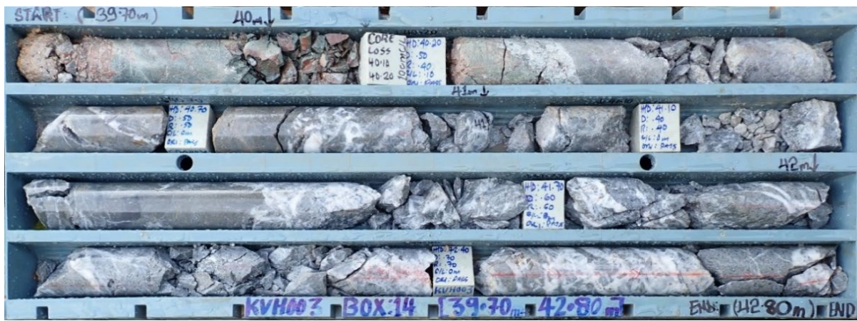
Figure 6: Drill core from the Kavasuki hole KVVH-03 (39.7-42.8 m) showing intense silica flooding and multi-phase quartz veining within hydrothermally altered host rock.
