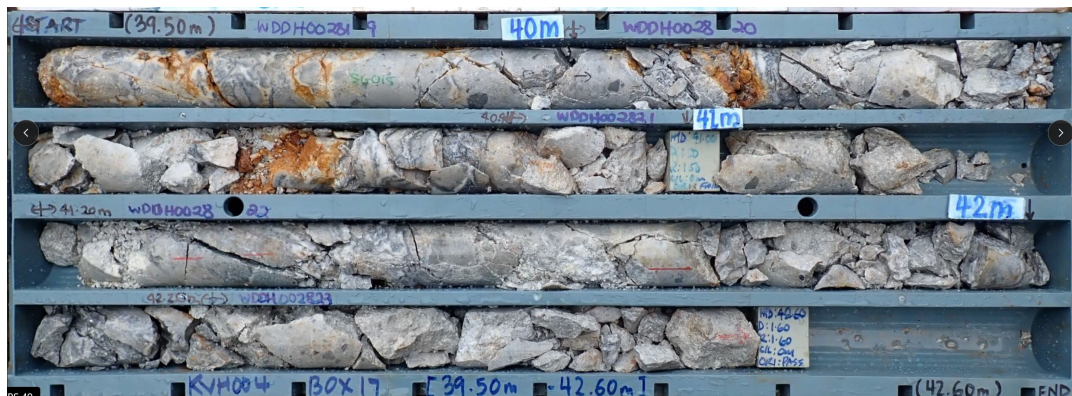
Figure 8: Drill core from KVH-04 illustrating crackle to mosaic brecciation with quartz-carbonate veining and fine sulphide mineralization.
