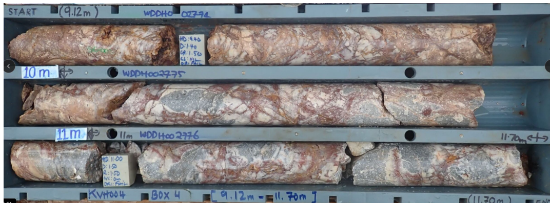
Figure 7: Drill core from KVH-04 showing intense silica flooding and multi-phase quartz veining with disseminated sulphides within a brecciated quartz matrix.
