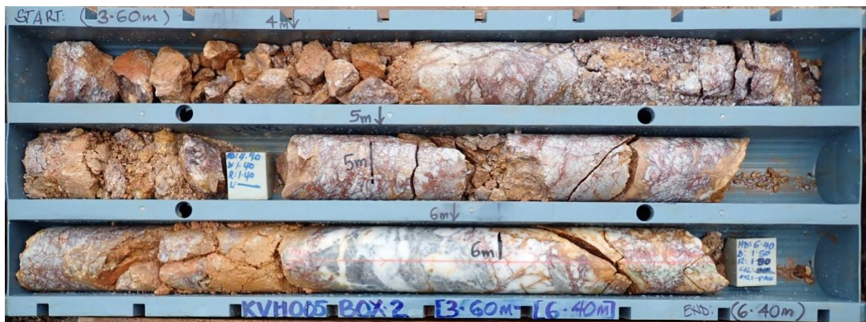
Figure 3: KVH-05 drill core (3.60–6.40 m) showing oxidized quartz–carbonate veining with associated hydrothermal breccia.
