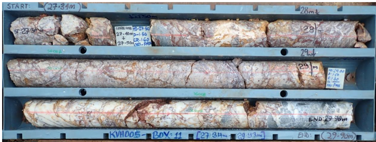
Figure 4: KVH-05 drill core (27.34–29.93 m) showing strong, continuous quartz–carbonate veining and localized hydrothermal brecciation.
