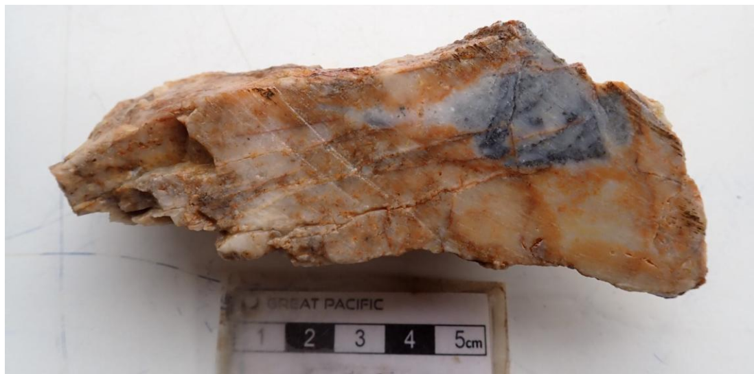
Figure 5: Rock-chip sample WDGs260242 collected northeast of the main Kargalio Vein showing quartz-silica-pyrite vein material associated with silica-sericite-pyrite alteration, late-stage silica overprinting and disseminated fine-grained sulphide mineralization.
