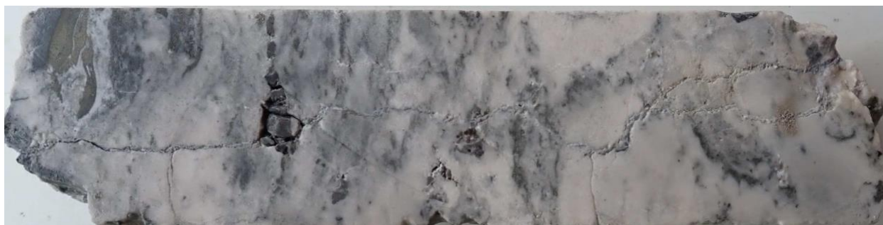
Figure 5: KAS-01 at 376.3 meters downhole as an example of intense alteration (Quartz-Sericite-Pyrite). Intense zones of alteration appear to be structurally controlled with strong alteration to the end of hole at 593.5 m.
