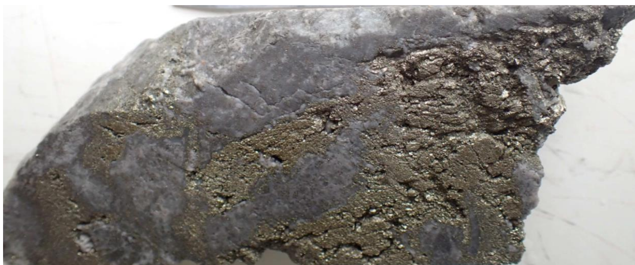
Figure 6: KAS-01 at 462.2 meters downhole as an example of semi-massive sulphide (Pyrite) zone. The sulphide-rich ground persisted to end of hole at 593.5 m.
