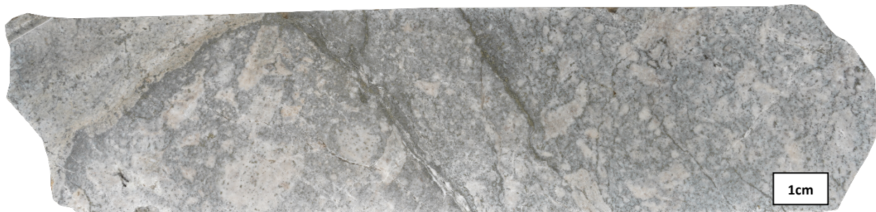
Figure 11: Pale grey silicified and argillic-altered volcaniclastic rock at 89.6 m, with fine disseminated pyrite and incipient crackle texture.
