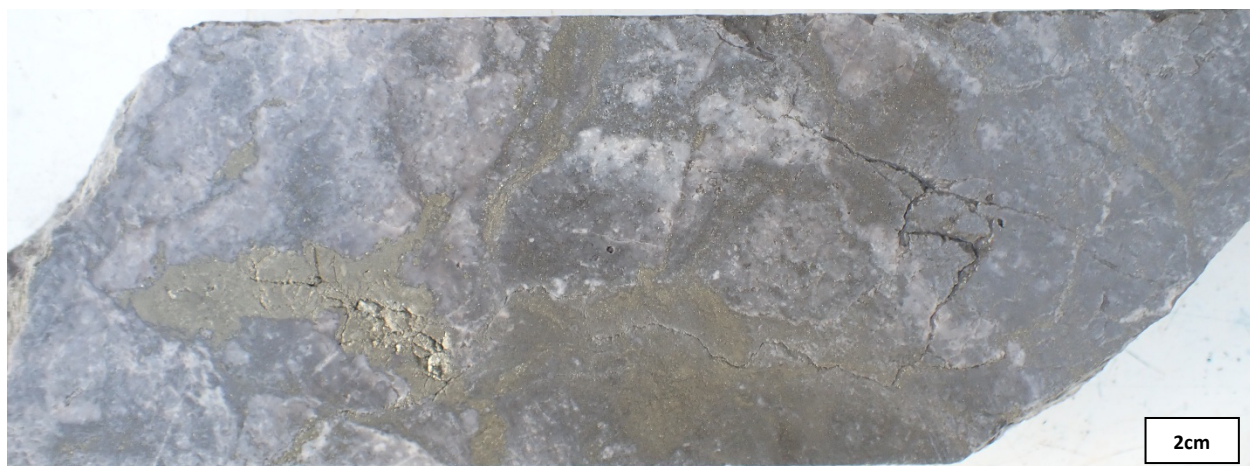
Figure 13: Crackle-brecciated, intensely silicified rock at 158.45 m, with pyrite forming irregular patches and veinlets, within the most sulphide-rich zone logged in the hole. Assay results are pending.
