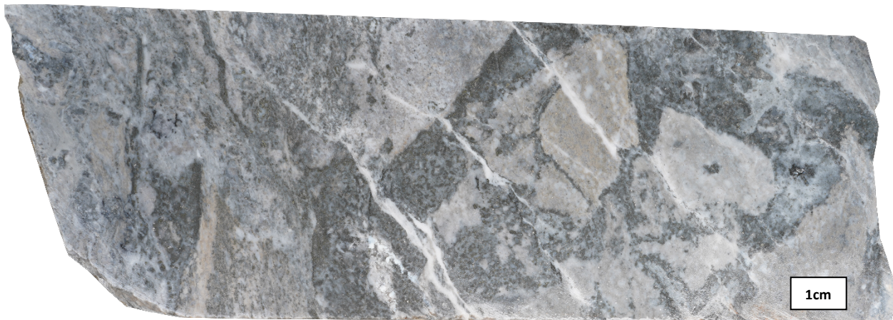
Figure 10: Brecciated, silica-overprinted sericite-altered crystal tuff at 69.4 m; fine dark sulphides and pyrite rim clasts and infill microfractures, cut by late white quartz-carbonate veinlets.
