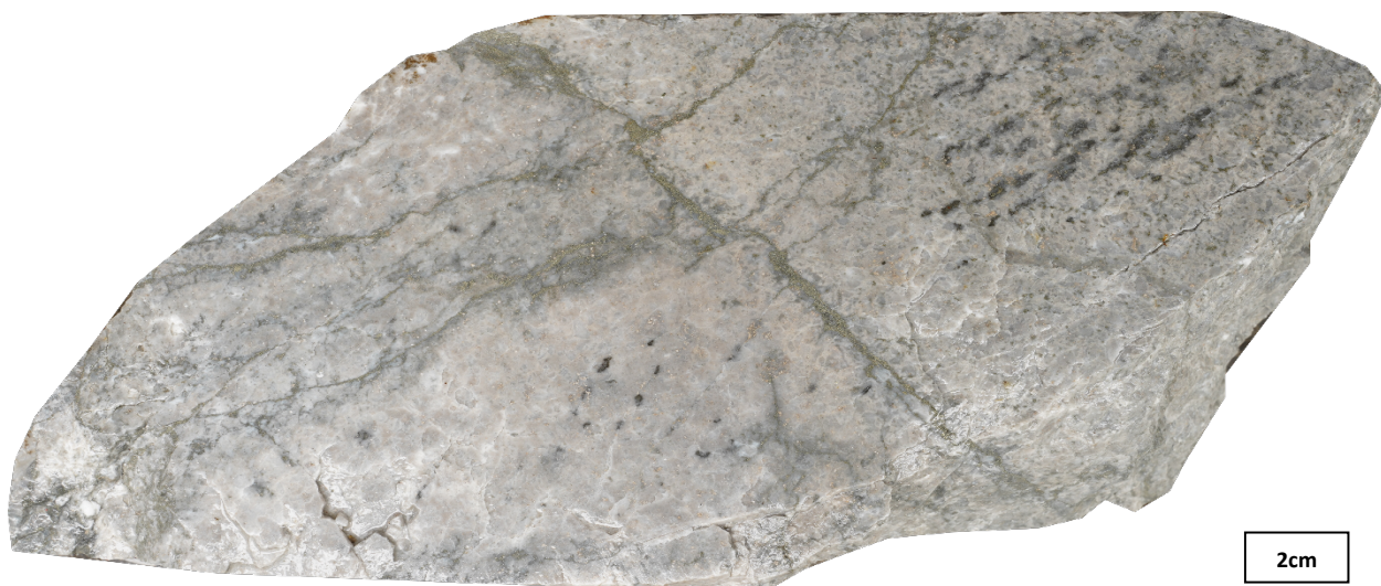
Figure 12: Silicified rock at 91.5 m cut by hairline pyrite stringers, with fine disseminated pyrite throughout.
