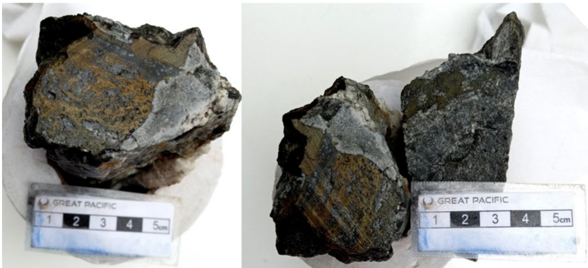
Figure 4: Cut hand specimens from the Magiabe West Vein discovery outcrop, displaying quartz–sulphide veining with visible semi-massive chalcopyrite and bornite mineralization. Scale bar in centimetres.
