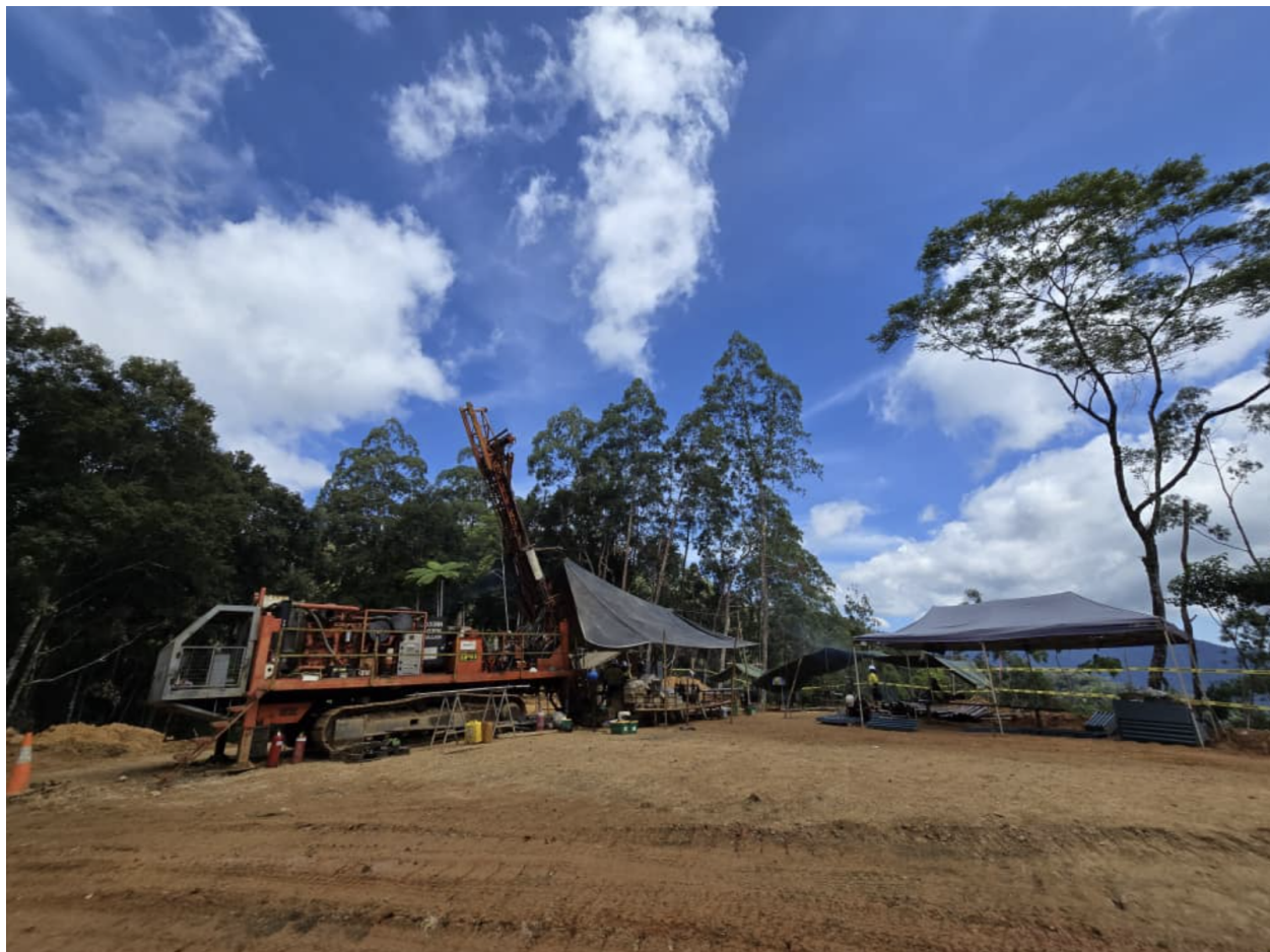
Figure 2: Photograph of drill rig (ZD01) established on the first drill pad (MGH001) at Magiabe.
