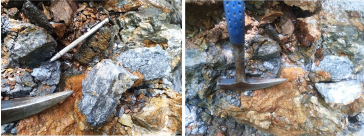
Figure 3: Magiabe West Vein discovery outcrop, showing brecciated quartz–sulphide mineralization within a silicified host. Visible sulphides occur along fracture surfaces and within the quartz matrix, consistent with a structurally controlled epithermal Au–Ag–Cu vein system.
